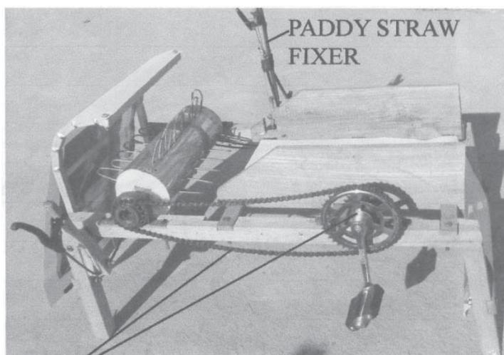
**Figure 3: Crank Shaft with the Iron Chain**
